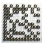
chemical etching may require extra manufacturing processes to apply the mask, etch the code, and remove the mask.
